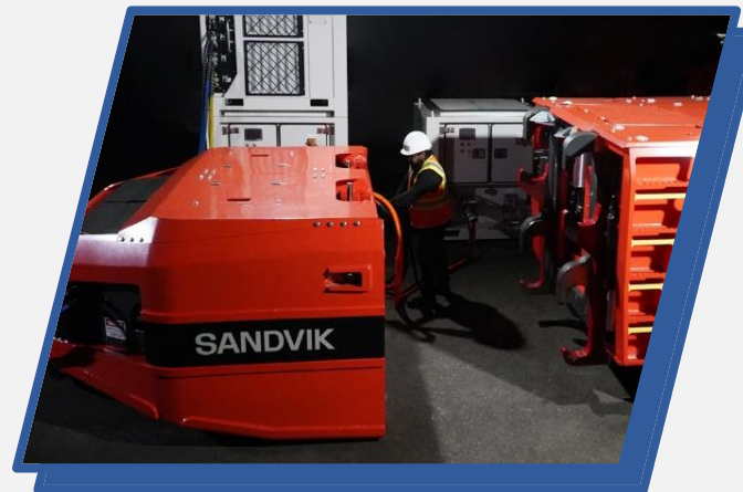
Sandvik: battery swap with onboard hydraulic device
