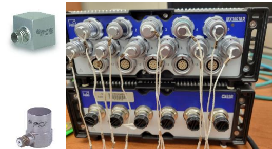
rugged dacq w/ accelerometers
