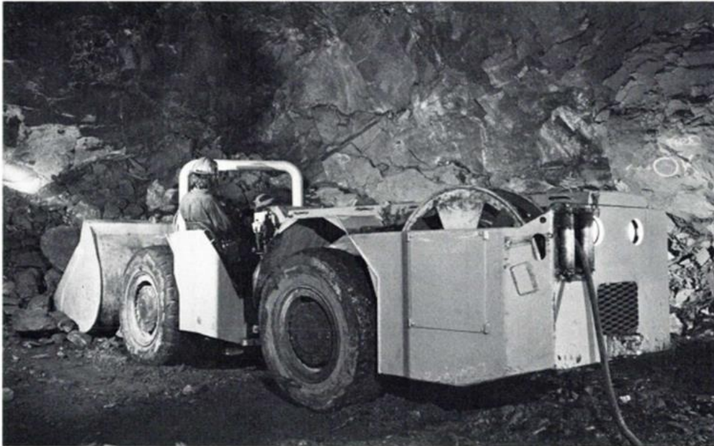
That's the new 2-yard electric scooptram , now in operation at Creighton mine. A new concept in load-haul-dump operation, the unit is operating in a cut-and-fill stope complex on the 6600 level.
